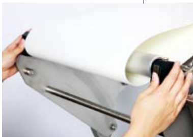
Conveyor belts are designed for easy, rapid removal for cleaning when required.
